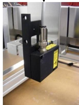
fig2: mounting laser sensor
